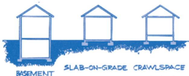
Others have more than one foundation design feature it is common to have a basement under part of the house and to have a slab-on-grade or crawlspace under the rest of the house. In these situations, a combination of different radon reduction techniques may be needed to reduce radon levels to below 4 pCi/L.
